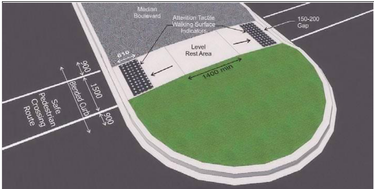
A good example of using curb ramps to facilitate access to an island.
